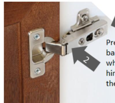
Press in on clip on back of hinge ① while pressing in on hinge ② to snap off the hinge.
